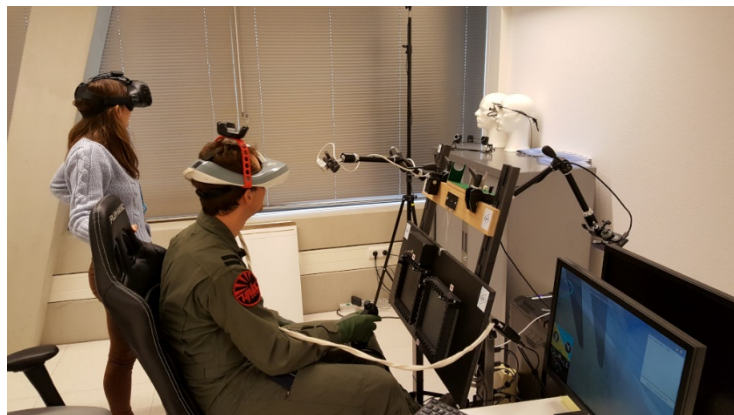
Figure 6: An Apache pilot flying the Virtual Cockpit during the third evaluation in the Cinoptics COBALT, while one of the researchers “hitch-hikes” along in the HTC VIVE.
